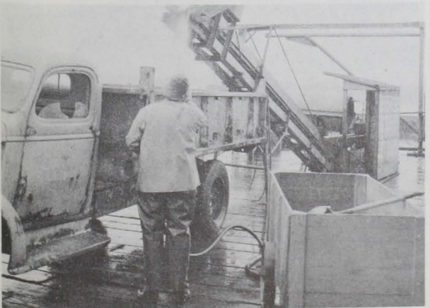
FIG. 9 - SCALE (40,000-POUND CAPACITY) FOR WEIGHING FISH.
