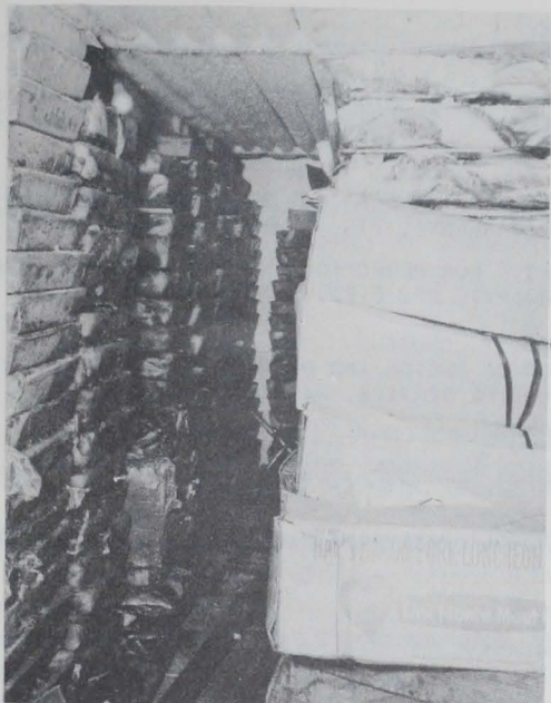
FIG. 26 - FROZEN STORAGE FACILITIES OF FUR FARMER AT BAY CITY, ORE. FISH PRODUCTS ARE OBTAINED FROM ASTORIA, NEWPORT, AND NEARBY GARIBALDI. THE PRODUCTS, IF NOT BAGGED, ARE FROZEN AND THEN ICE GLAZED TO PREVENT DESICCATION AND OXIDATION.
