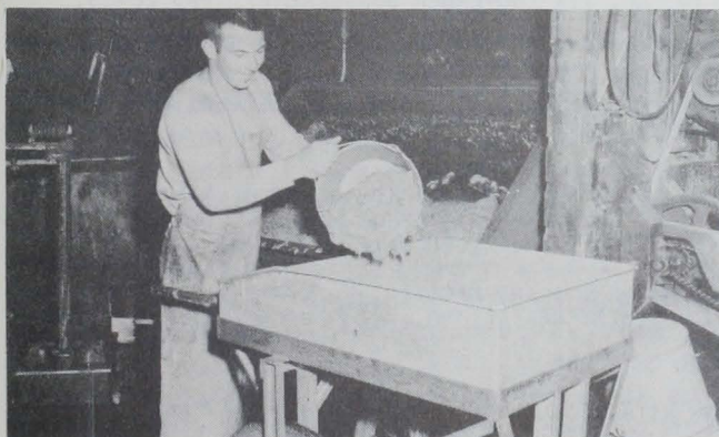
FIG. 28 - LOADING GROUND-UP FISH MIXTURE INTO CART. THE MIXER BEHIND THE WORKMAN IS RUN BY A 5-HORSEPOWER, 3-PHASE MOTOR.
