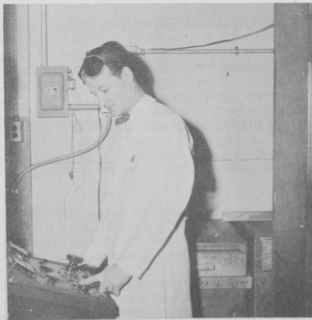
FIG. 1 - DETERMINING THE "BONE-CONTENT" OF FISH STICKS, BLOCKS, OR FILLETS BY USE OF X-RAY FLUOROSCOPY. THE OPERATOR IS ADJUSTING THE X-RAY CONTROL PANEL.
