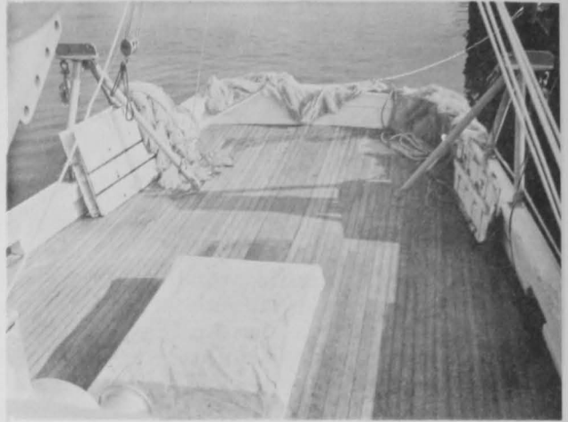
Fig. 5 - After deck view showing trawl davits. Trawling may be done either with these davits or with the "Florida-type" trawling boom.
