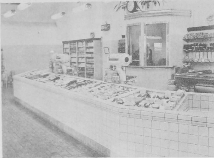
Retail store in St. Louis, Mo., fluorescently illuminated with tiling and stainless steel trimming throughout, including interior and exterior of cases. Transparent lucite covers on cases.
