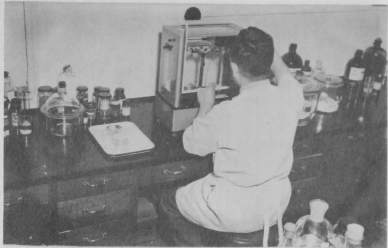
Fig. 2 - Weighing fish samples for the determination of moisture.
