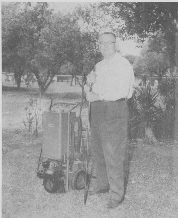
Experimental pump and probe designed to introduce fish oil nematocides into the ground surrounding the roots of citrus trees threatened by the "spreading-decline" nematode.
