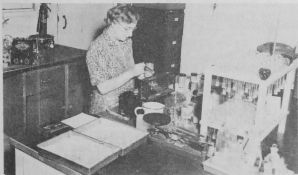
Fig. 2 - Microbiological assay of fish meal samples for B vitamin.
