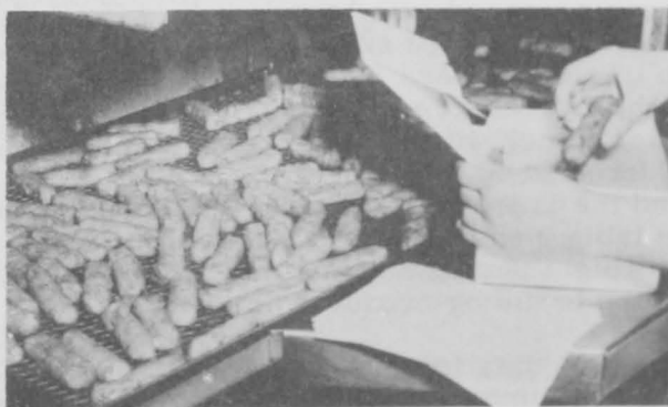
Cooked fish sticks being packed in institutional packages prior to freezing and storage.
