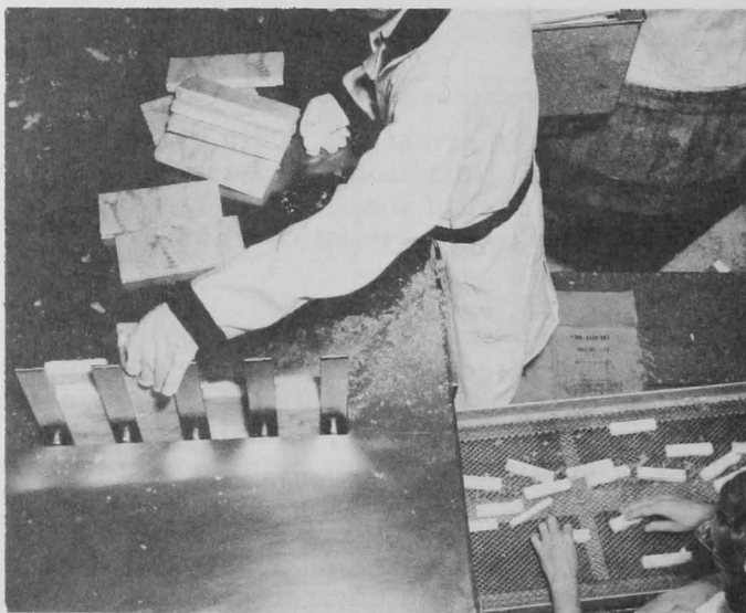
Frozen fish fillet blocks being cut into uniform fish sticks in a modern conveyor-belt-equipped plant.
