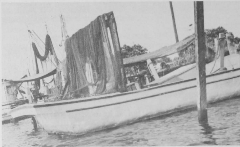
Stern view of shrimp skiff showing shrimp trawl spread for drying. Note overhang of platform used to shoot and haul in the net.
