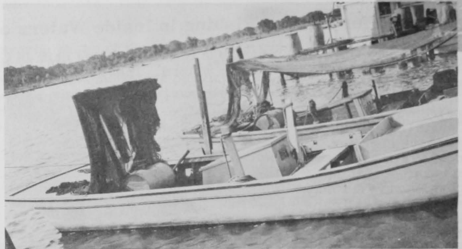
Another view of the shrimp skiff showing the small frame on the port side next to the seat. This frame is used on a number of boats. Inserted in the two holes are two small pieces of wood or planks (2-2½ feet long) extending out over the water to support the cod end with the catch and hold it open so that the catch may be brailed out with a small hand net.
