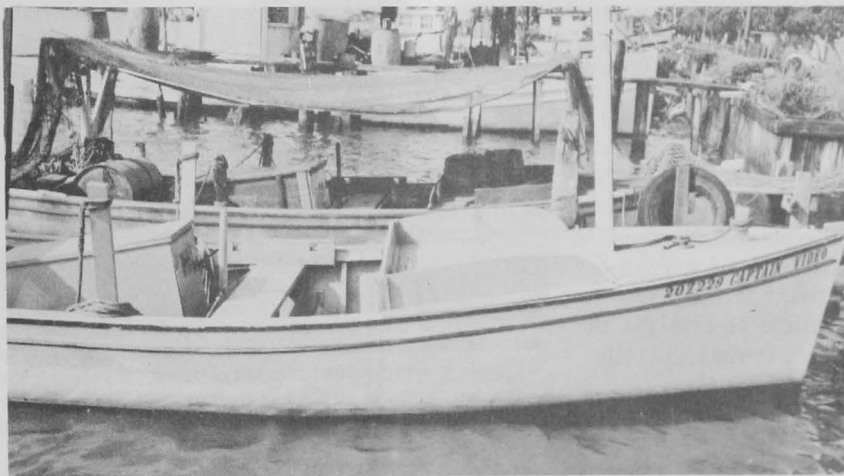
A side view of the new type of skiff used for shrimp fishing in the inside waters of the Gulf of Mexico. Note sorting platform in place near bow.
