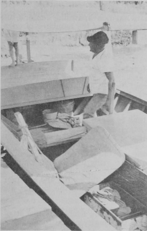
A view of the bow of a shrimp skiff showing the sorting platform in place.
