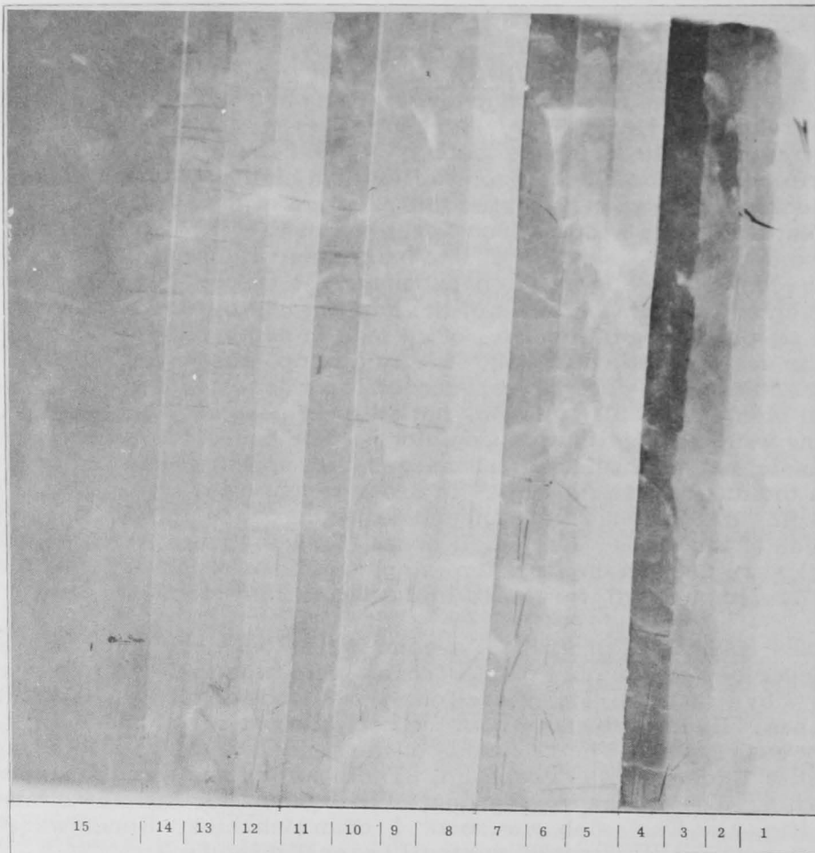
Fig. 1b - Radiograph of fillet block taken from the top view showing bones. Although the bones were inserted at indicated heights, the radiograph shows that they necessarily were not inserted in the uniform arrangement shown in the sketch above. Numbers show the steps as sketched above.
