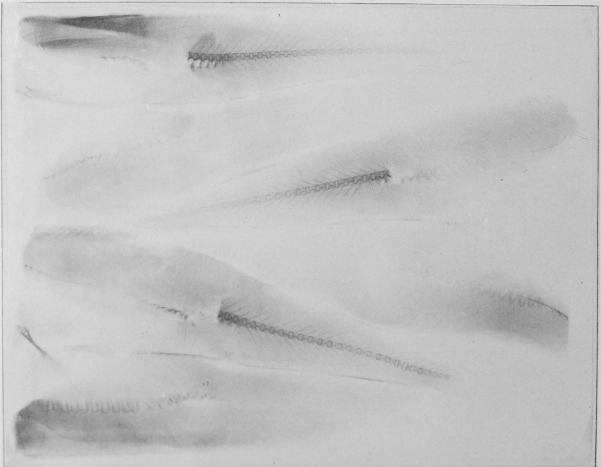
Fig. 7b - Radiograph clearly reveals the bones in the split whiting butterfly portions.
