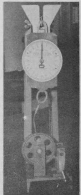
Fig. 4 - Tenderometer used for measuring texture changes in the meat of fish.
