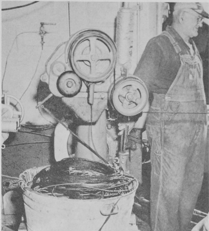
Fig. 28 - A side view of the Japanese long-line hauler in operation.
