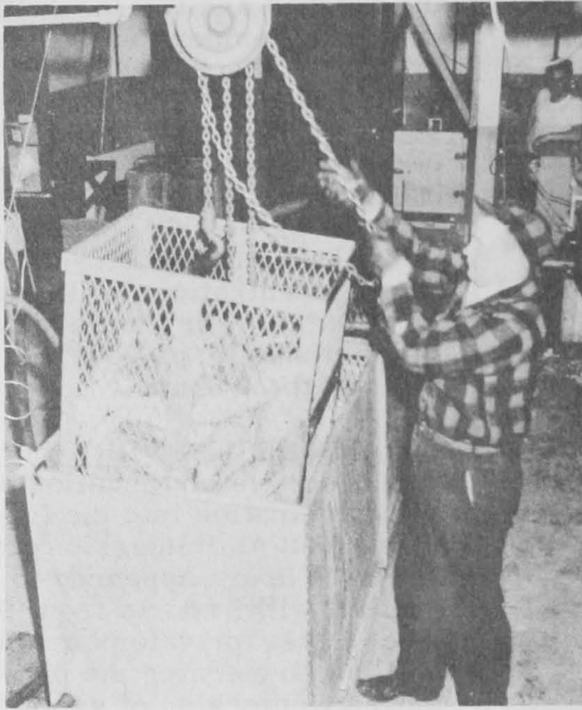
Fig. 3 - Hoisting defrosted round fish from the thawing tank.
