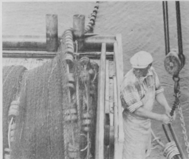
FIG. 13 - THE PURSE RINGS ARE PULLED OFF THE CLOTHESPIN BY THEIR BRIDLES, ONE BY ONE, AND GO BACK OVER THE ROLLER AND ON TO THE DRUM ALONG WITH THE PURSE LINE AND THE OTHER PARTS OF THE SEINE.
