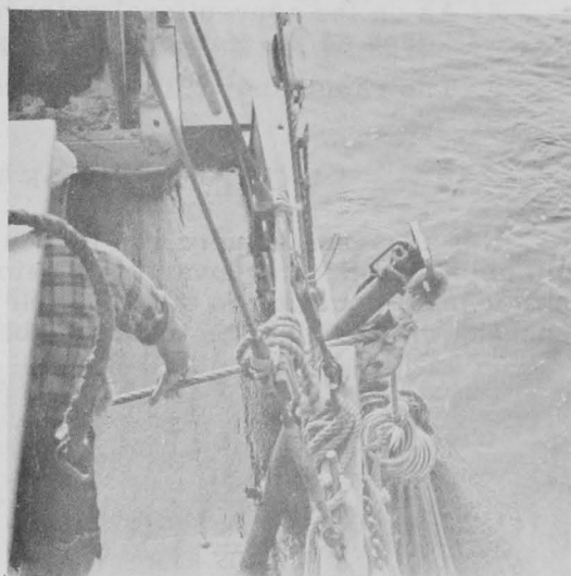
FIG. 11 - THE PURSE RINGS ARE DRAWN UP TO THE DAVIT.
