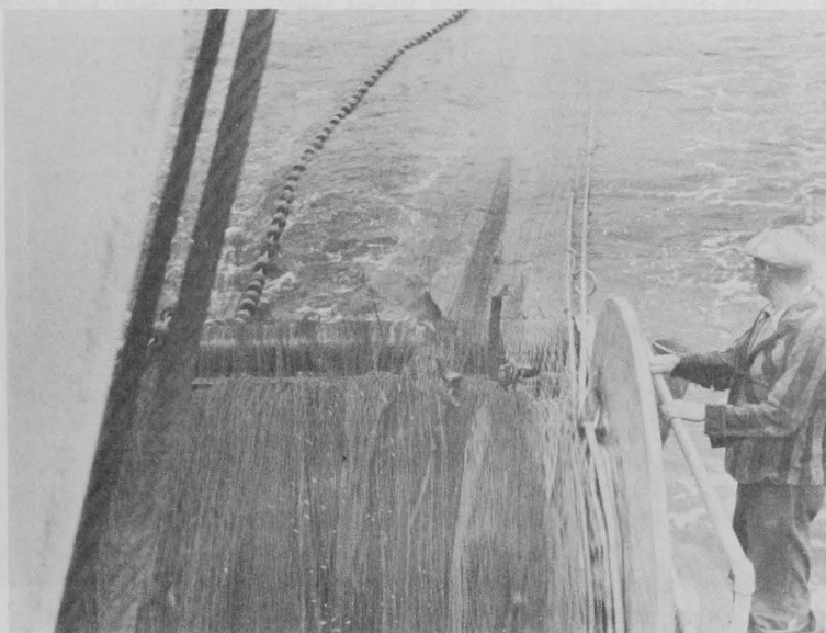
FIG. 5 - A SET IS STARTED AS THE SEINE UNWINDS RAPIDLY FROM THE DRUM. THE ROLLERS OF THE SPOOLER ARE REMOVED FROM THEIR SOCKETS WHILE THE SEINE IS BEING SET. ONE OF THESE ROLLERS CAN BE SEEN STOWED JUST BEHIND THE FISHERMAN'S RIGHT WRIST.
