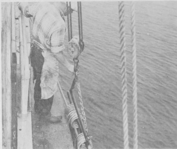
FIG. 12 - THE PURSE RINGS ARE THREADED ONTO THE "CLOTHESPIN" AND HOISTED INTO POSITION AT DECK LEVEL.
