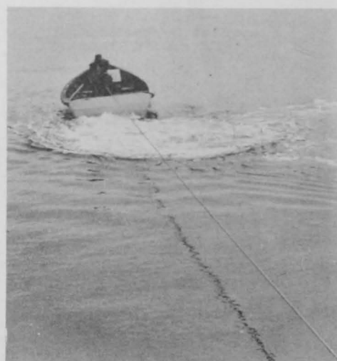
FIG. 9 - THE SKIFF TOWS THE VESSEL AWAY FROM THE SEINE DURING PURSUING AND HAULING
