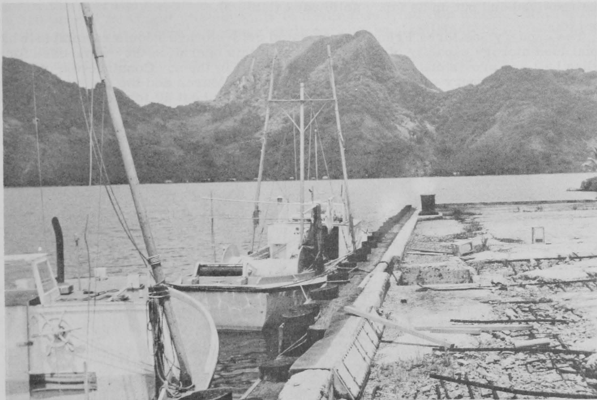
Fig. 4 - Salmon gill-net boats at the Oil Dock, Pago Pago Bay, rigged for tuna fishing with trolling outriggers and with long lines reeled up on the net drums.
