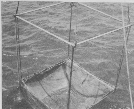
FIG. 3 - TRAP LIFT NET FRAME RAISED IN POSITION FOR REMOVAL OF CATCH WITH A DIP NET. SIDES HAVE BEEN LOWERED.
