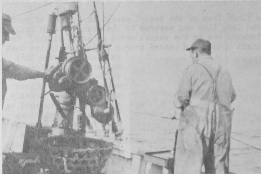
FIG. 6 - HAULING LONG LINE WITH JAPANESE-TYPE LINE HAULER. THE MAIN LINE IS AUTOMATICALLY COILED IN THE BASKET BELOW THE MAIN HAULING SHEAVE.
