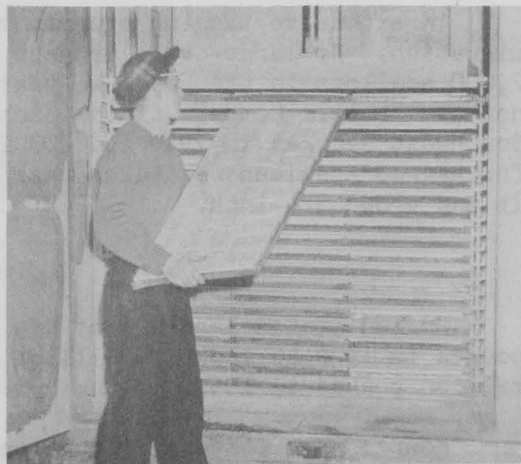
FIG. 11 - PLATE-TYPE QUICK FREEZER IS USED BY A LEADING NEW BEDFORD FIRM FOR FREEZING CONSUMER PACKAGED SCALLOP MEATS.
