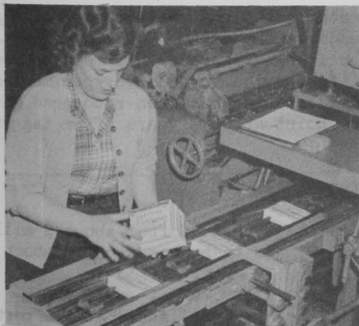
FIG. 10 - CLEANED RAW SCALLOP MEATS OR PRE-COOKED SCALLOPS ARE PACKED IN CONSUMER-SIZE (10 OZ.) PACKAGES PRIOR TO FREEZING. AUTOMATIC WRAPPING AND SEALING MACHINE IN OPERATION.
