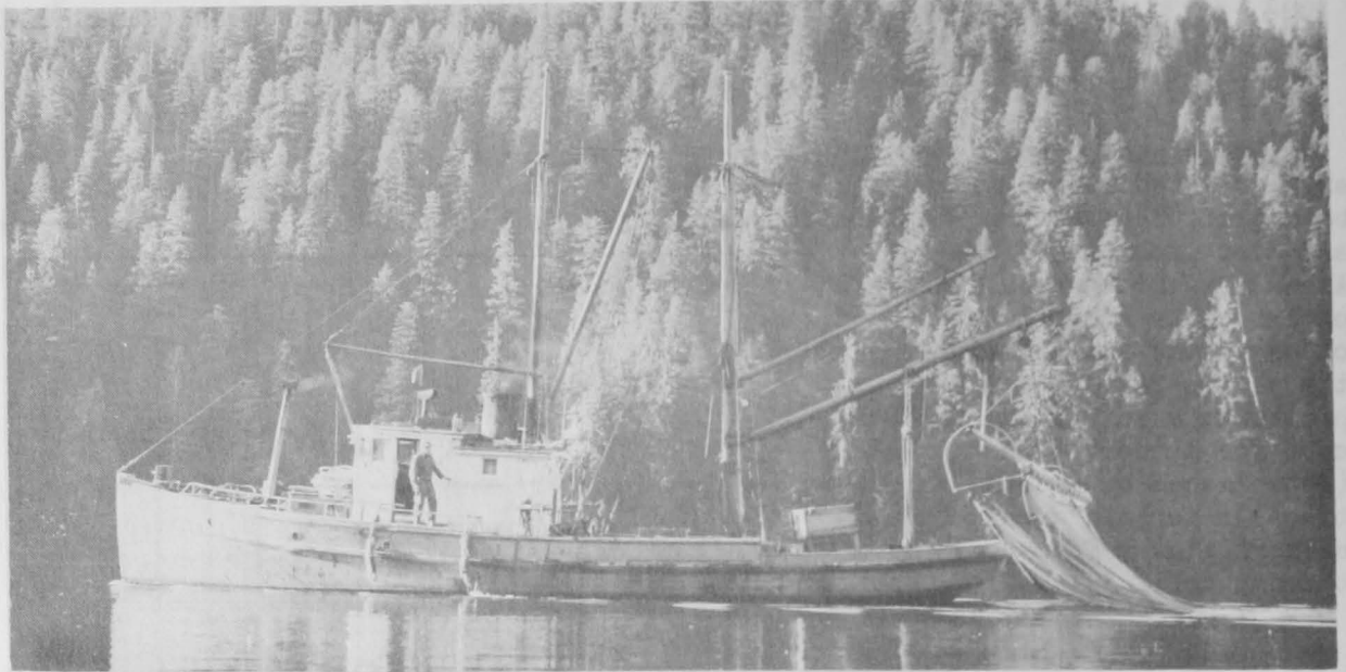
FIG. 2 - TYPICAL ALASKA SHRIMP TRAWLER PREPARING TO "SET" THE BEAM TRAWL.
