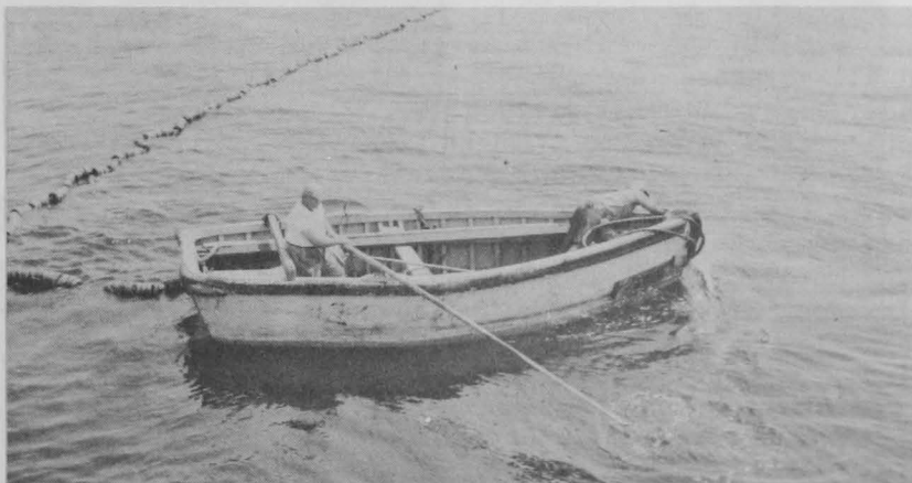
FIG. 7 - SKIFF MAN MAKING FAST THE EXTENSION PURSE LINE TO END OF SEINE.
