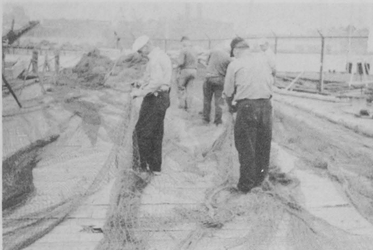
FIG. 16 - HANGING SEINE. LACING TOGETHER WEB STRIPS IN MIDDLE OF SEINE.
