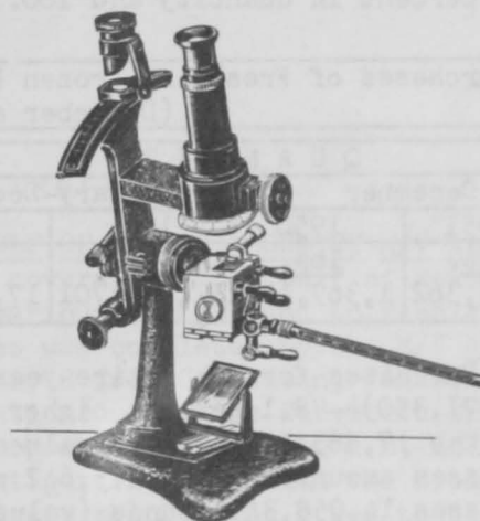
REFRACTOMETER USED FOR DETERMINING REFRACTIVE INDEX OF FREE OIL IN CANNED SALMON.
