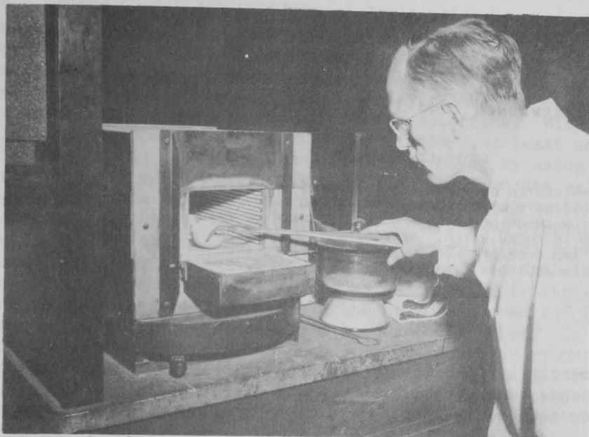
TECHNOLOGIST PREPARING CRUCIBLES FOR ASH DETERMINATIONS OF CONDENSED FISH SOLUBLES AT THE SERVICE'S COLLEGE PARK TECHNOLOGICAL LABORATORY.
