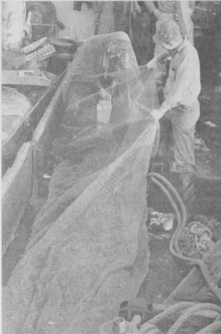
FIG. 2 - IN ORDER TO MEASURE THE MESHES OF THE EXPERIMENTAL COD END IT WAS NECESSARY TO CRAWL INSIDE THE COVER.
