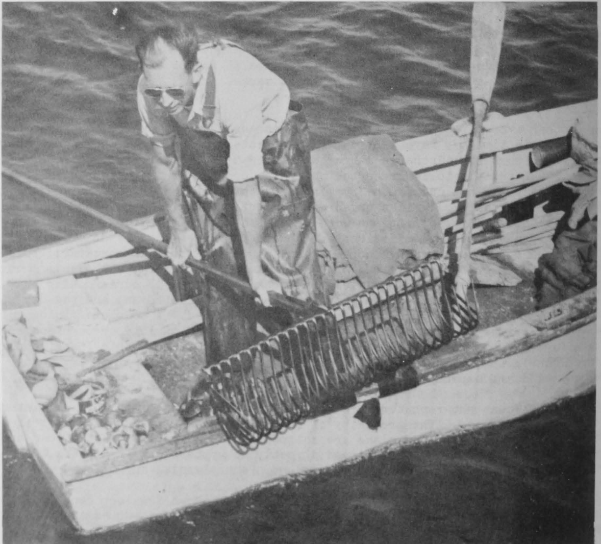
FIG. 7 - BULL RAKES ARE EQUIPPED WITH SECTIONAL STALES OR HANDLES FOR FISHING IN WATER 20 TO 25 FEET DEEP.
