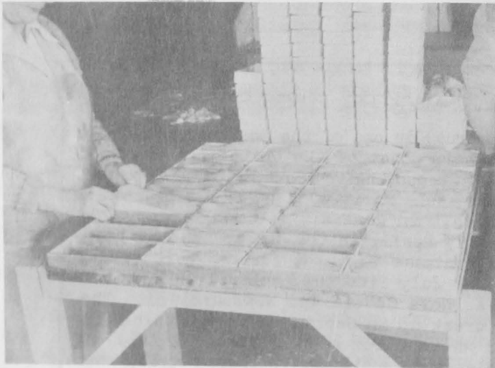
PREPARING FISH FILLETS FOR FREEZING IN ONE-POUND UNITS IN A WEST COAST FISH-PROCESSING PLANT.
