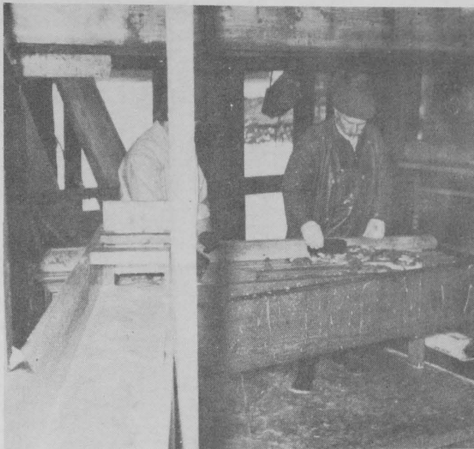
FIG. 4 - ANOTHER VIEW OF THE DRAINING TABLE SHOWS THE VISCERA FLOWING DOWN THE CHUTE, THROUGH THE TRAP DOOR, AND ONTO THE DRAINING TABLE.
