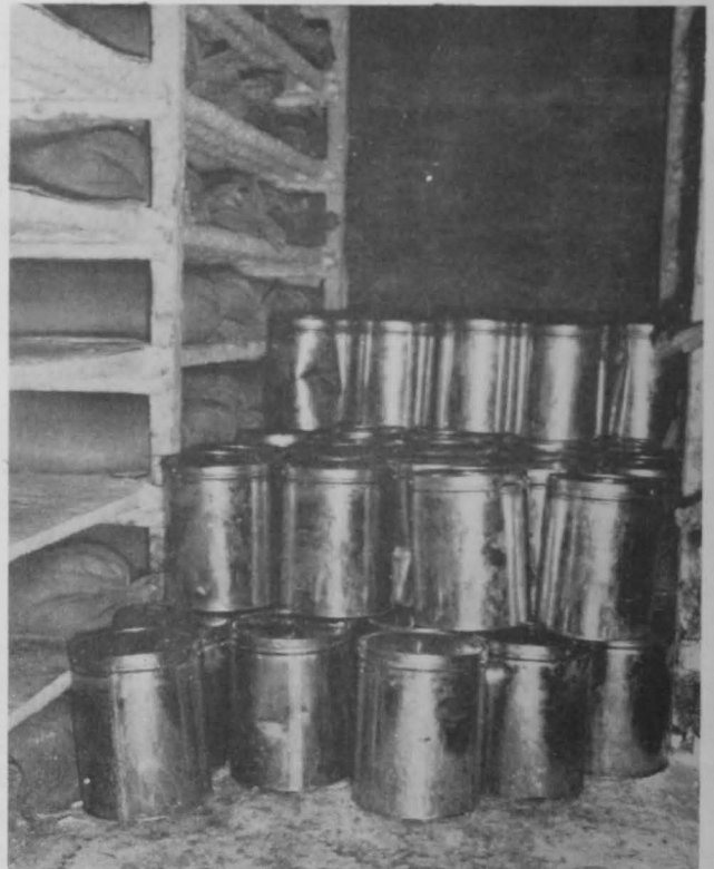
FIG. 8 - THE SACKS OF VISCERA ARE LYING ON THE FREEZER PLATES (LEFT) WHERE THEY ARE NORMALLY FROZEN SOLID IN 24 HOURS; THE CANS CONTAINING THE EGGS WERE FROZEN WHILE STACKED ON THE FLOOR.
