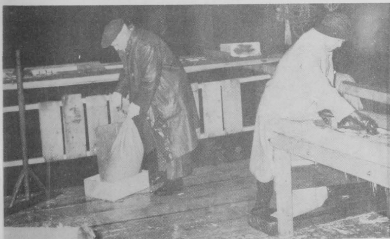
FIG. 5 - THE DRAINED VISCERA ARE SACKED (RIGHT) AND THE BUR-LAP BAG IS WIRE-TIED (CENTER).
