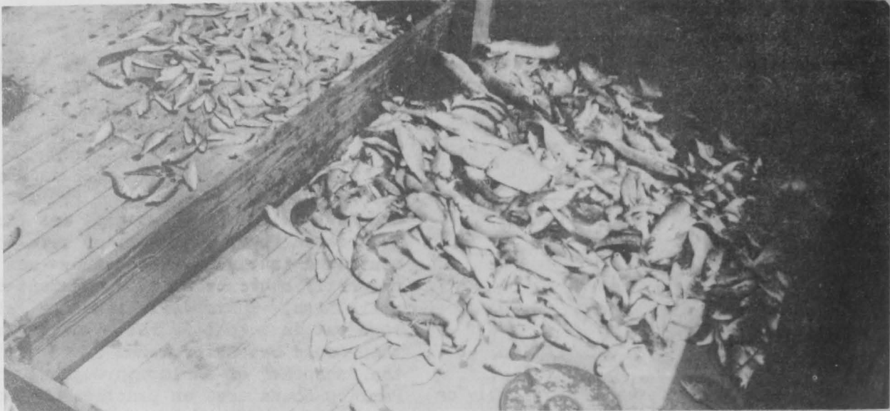
FIGURE 4 - WHEN THE NET WAS LIFTED, THE CONTENTS OF THE COVER BAG (UPPER CHECKER) AND THE COD END (LOWER CHECKER) WERE DISCHARGED INTO SEPARATE COMPARTMENTS ON DECK. SMALL FISH IN UPPER COMPARTMENT WERE RELEASED.
