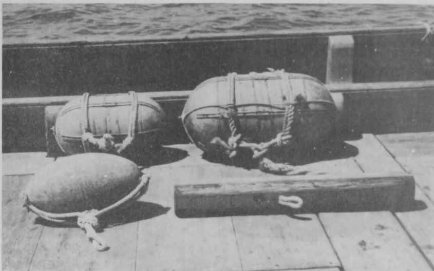
FIGURE 6 - FLOATS USED IN THE HAWAIIAN LONG-LINE FISHERY. THE ALUMINUM OXYGEN TANKS AND THE GALVANIZED METAL FLOATS ARE USED TO SUPPORT THE MAIN LINE AT THE CENTER OF A BASKET. THE WOODEN FLOAT IS FASTENED TO THE FLAGPOLE AND IS ATTACHED AT THE "HEAD" OF THE BASKET.
