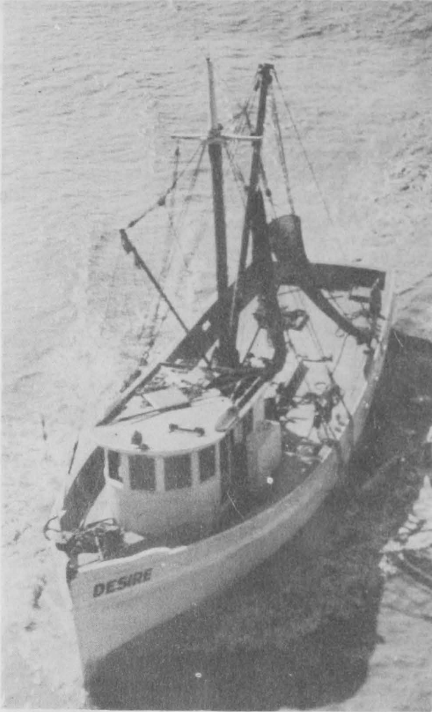
A TYPICAL LOUISIANA OFFSHORE TRAWLER OF ABOUT 60 FT. OVER-ALL LENGTH AND 16 NET TONS
