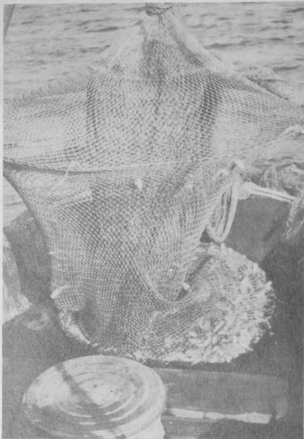
NEW EXPERIMENTAL SHRIMP TRAWL, INSIDE OF TESTING BAG, WHICH COLLECTED IMMATURE FISH THAT WERE ABLE TO PASS THROUGH THE INSIDE NET.
