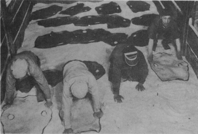
KENCHING SEALSKINS, ST. PAUL ISLAND, ALASKA. SKINS ARE SALTED AND PLACED IN BINS FOR TEN DAYS OR LONGER, THEN ROLLED FUR SIDE OUT IN BUNDLES, PACKED IN BARRELS, AND SHIPPED TO ST. LOUIS FOR DRESSING, DYEING, AND SALE AT PUBLIC AUCTION.
