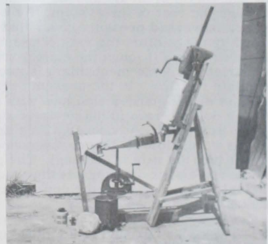
Fig. 1 - Experimental equipment used to convert raw fish into thiaminase-free press cake.
