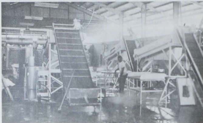
Fig. 3 - The most modern shrimp plant in Panama City has two sorters--one for large and the other for titi shrimp.
