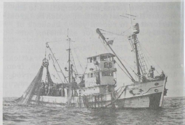
A Korean mackerel seiner equipped with a power block for hauling in the huge net. This is an indication that Korea is modernizing its fleet.
