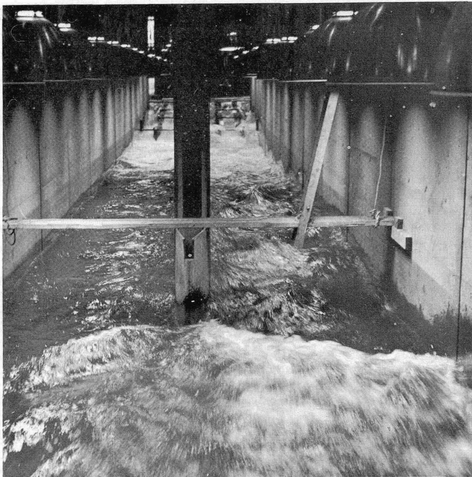
FIGURE 5.—View of choice area and channels showing 6 f.p.s. flow on left and 8 f.p.s. flow on right. Note positions of standing waves. Platform above downstream end of channels was used to check water velocities and was removed during the tests.
