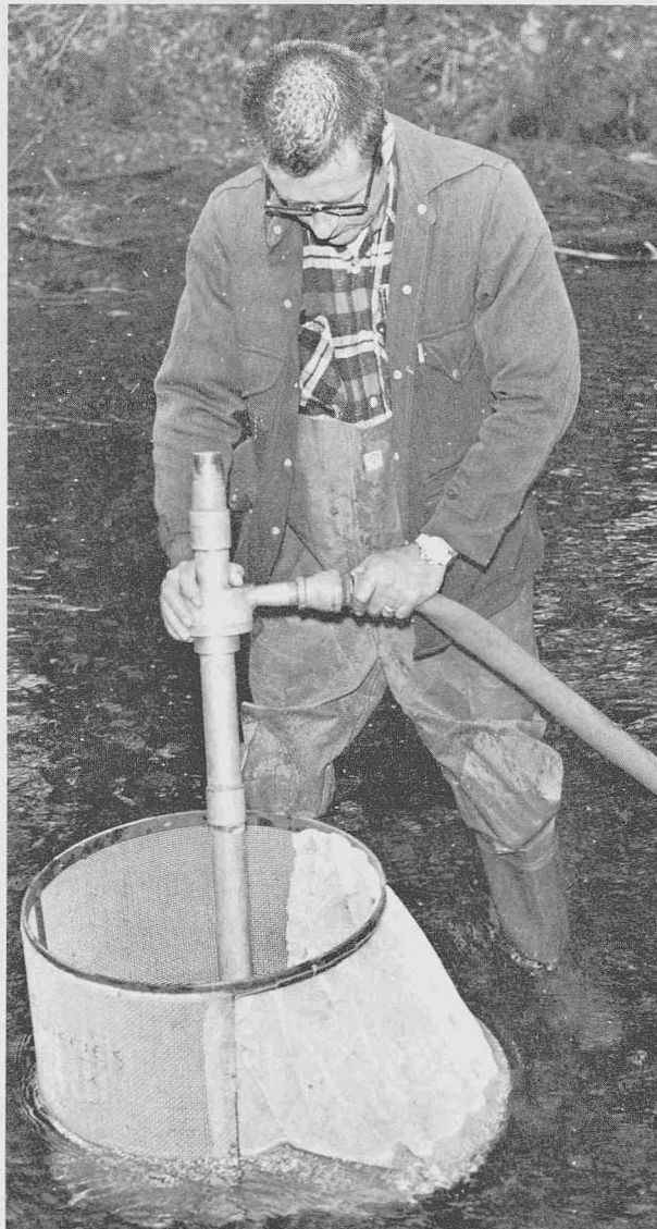
FIGURE 1.—Collecting pink salmon eggs or larvae with hydraulic sampler.
