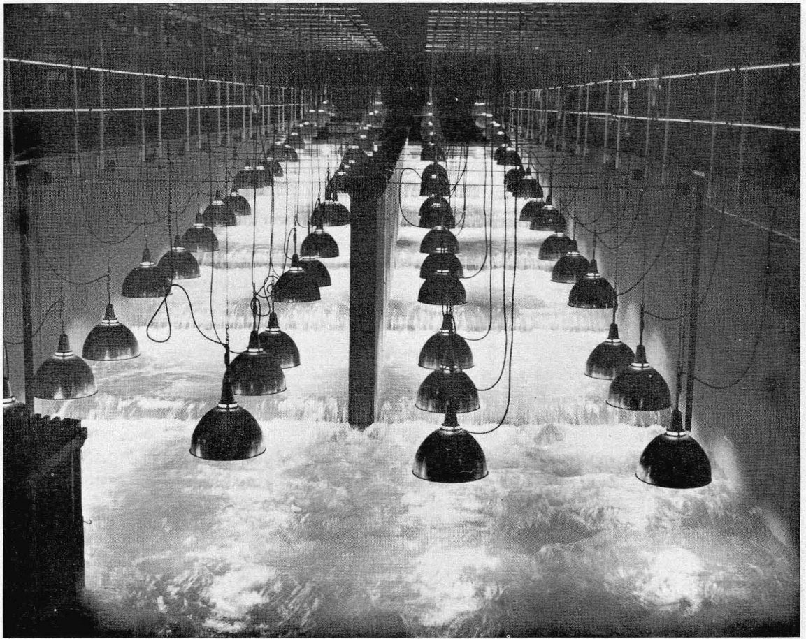
FIGURE 6.—Identical type-1 fishways with 1,000-watt mercury-vapor lights in place. Each light was 6 feet from the water surface.
