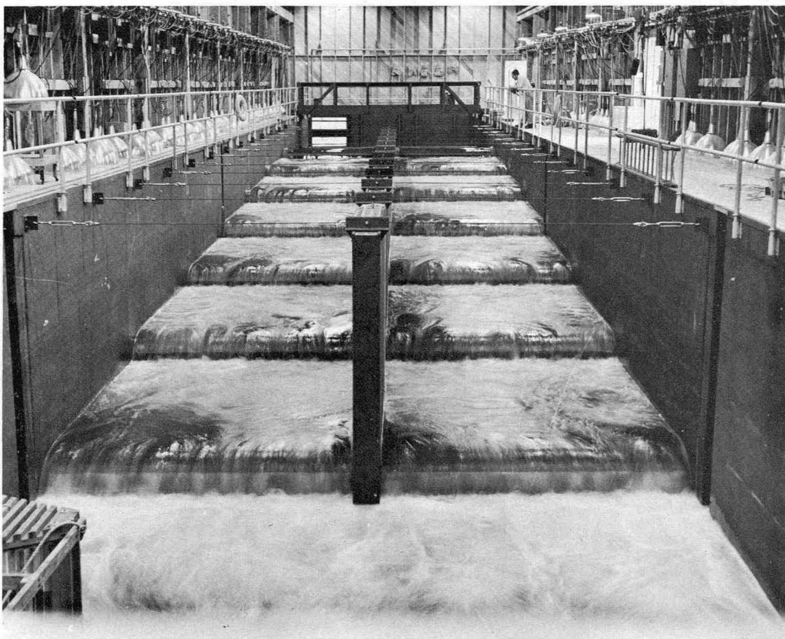
FIGURE 9—Identical type-1 fishways used to test for equal passage times in the north (on the left) and south channels. The mercury-vapor lamps were removed to provide an unobstructed view of the fishways.
