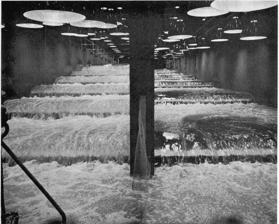
FIGURE 10.—A type-2 fishway on the left and a type-1 on the right. Note the greater turbulence in the type-2 fishway.
