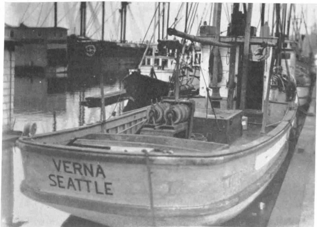
FIGURE 21.—Stern view of trolling boat. Note the two hand-operated gurdies and the lead-in blocks directly over them and on both gunwales. The two main poles may be seen at the sides of the mast.
