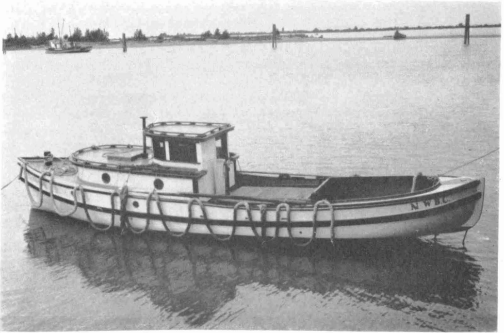
FIGURE 6.—Modern Fraser River gill-net boat. These round-bottomed motorized boats are very seaworthy, being relatively independent of the vagaries of the weather. They are more efficient than the skiffs in use during the earlier years, or the round-bottomed boats in use before motors were installed.
