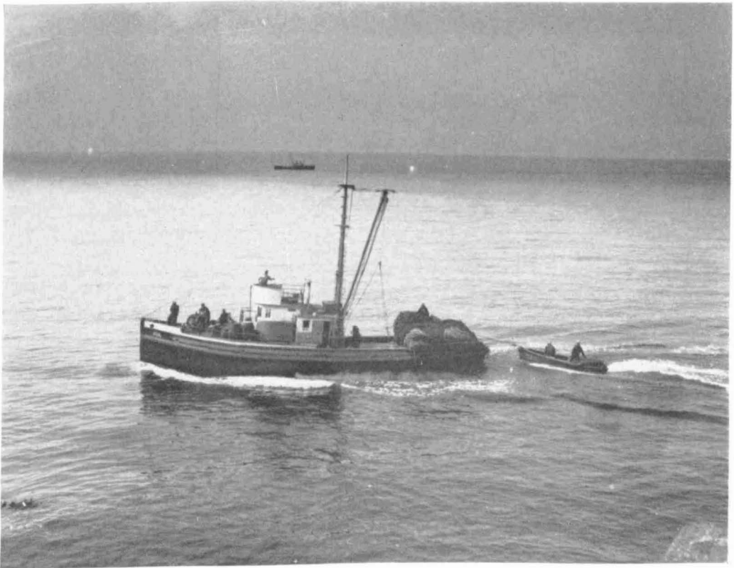
FIGURE 14.—A gasoline-powered purse-seine vessel built in 1920, of 27 net tons. The ports forward indicate that the crew's quarters are in the forecabin. The "flying bridge" with steering wheel and controls, atop the wheel house, are visible. A seine skiff is towed astern.
