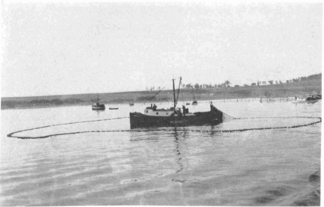
FIGURE 13.—An early Puget Sound purse-seine vessel, of 12 net tons, built in 1909. Note the large house on deck containing the crew's quarters, and the outside steering wheel in front of the house.
