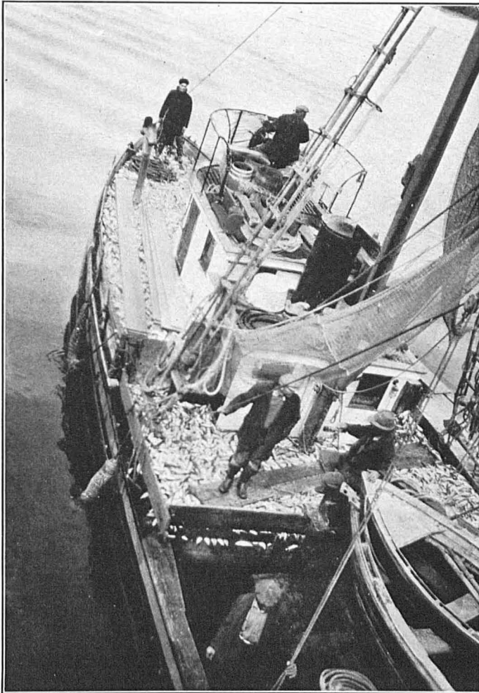
FIGURE 11.—The purse boat Lemes II , decks awash, at Pillar Bay, with a "deck load" of herring from Douglas Island (area 20). Note the outside setting wheel atop the wheelhouse. This is being installed on all of the new boats for quick and easy maneuvering while seining. Taken July, 1929
