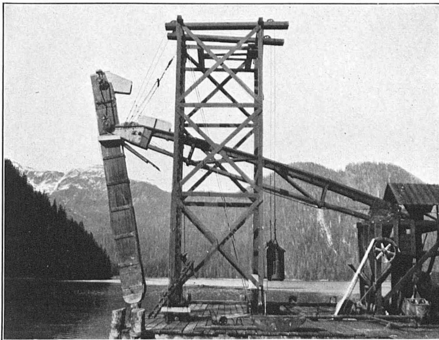
FIGURE 25.—Close-up of the endless-chain bucket fish elevator shown in Figure 24
