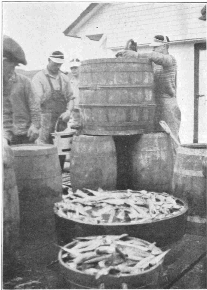
FIGURE 41.—Repacking at Dutch Harbor. Brine is being mixed in the large tierce and drawn off through a spigot. The herring that are to be used in filling up the barrels are being washed in the half tierce in the foreground.
