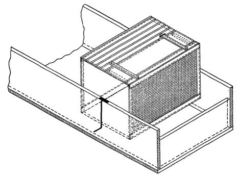
FIG. 2.—Apparatus for cleaning mussels preparatory to canning or other preservation process. (Drawn for the author by Prof. L. C. Harrington.)
