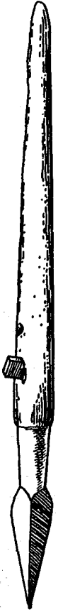
FIG. 3.—Hand pick used for making sockets in gravelly bottom for insertion of shibi.
