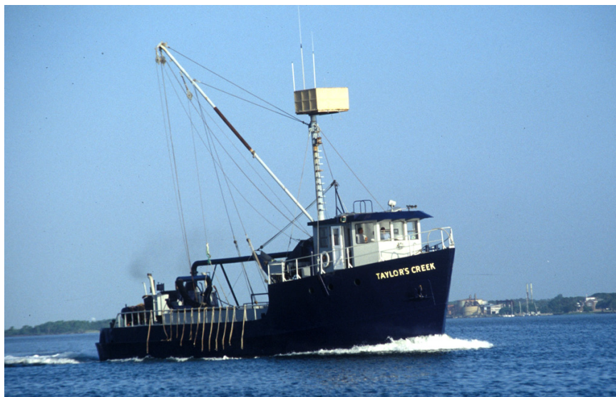
Figure 4.— F/V Taylor’s Creek , 87-ft long, began her career in Beaufort, N.C., as a purse-seiner for the reduction fishery. She moved to Northern Neck, Va., and began fishing with the “snapper rig” fleet in 1998. Photo credit: WBO.
