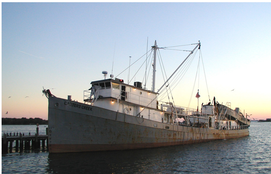
Figure 6.— F/V Carter's Creek is a 135-ft vessel which unloads Atlantic menhaden at Reedville, Va., for both bait and reduction. She began her service as a menhaden reduction vessel in the late 1950's, was converted to participate in various dredge and trawl fisheries in the 1970's, then was converted back to a menhaden purse-seiner in 2005. Photo credit: JWS.
