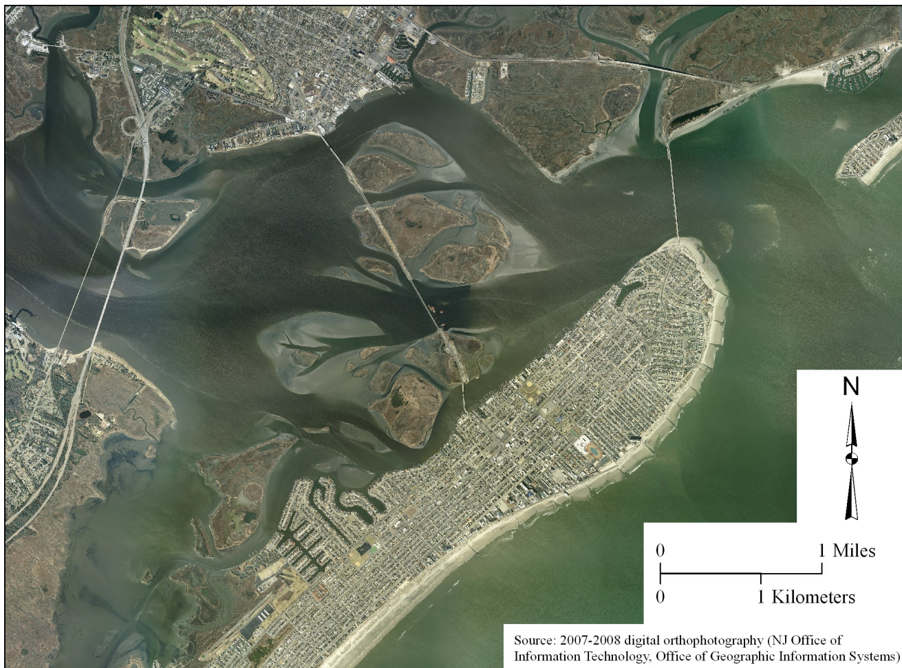
Figure 6.—Aerial view of Great Egg Harbor, portraying the submarine and subaerial morphological features of the flood-tide delta and the shoals and channels associated with the riverine system.
