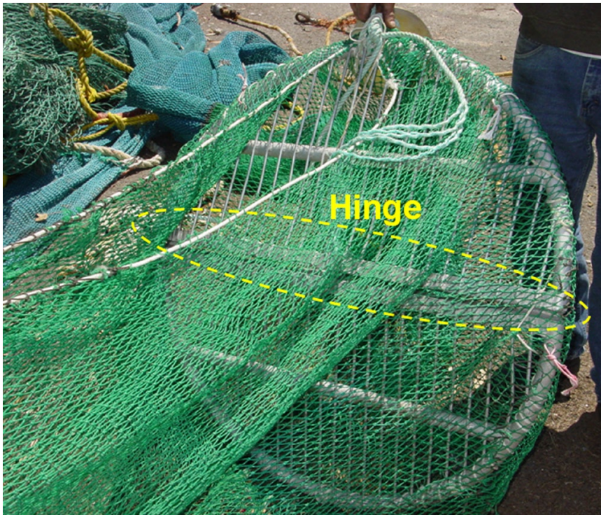
Figure 10.—Photograph of a hinged, or folded, rigid-grate BRD. Credit: Adam Fridmodig, CDFG.
