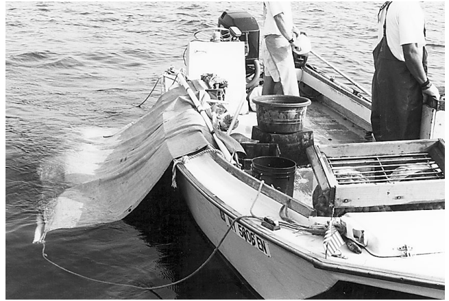
Figure 41. — Tide sheet used to pull quahog boat away from rake, Raritan Bay, N.Y., 1998. Photograph by C. L. MacKenzie, Jr.
