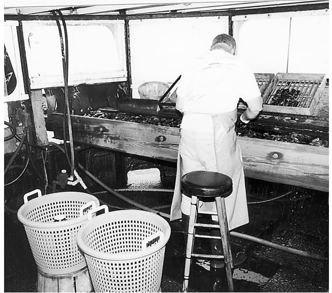
Figure 28. — Picking quahogs from “trash” moving along conveyor belt on hydraulic escalator dredge boat, Great South Bay, N.Y. Fisherman tosses the quahogs into hand sorters on the far side of the belt, 1998. Photograph by C. L. MacKenzie, Jr.
