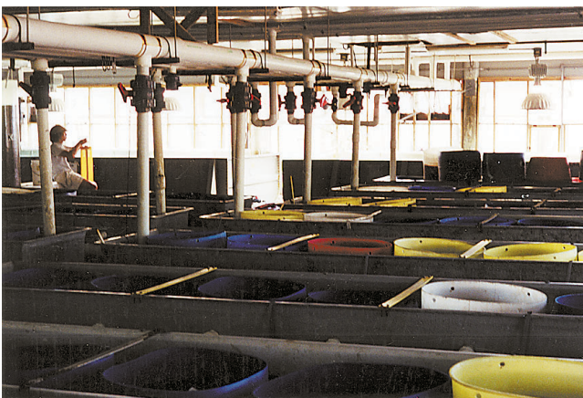
Figure 97. — Upweller tanks used to grow quahogs from 1-2.4 millimeters. Sea Perfect hatchery, Folly Beach, S.C. Photograph by V. G. Burrell, Jr.
