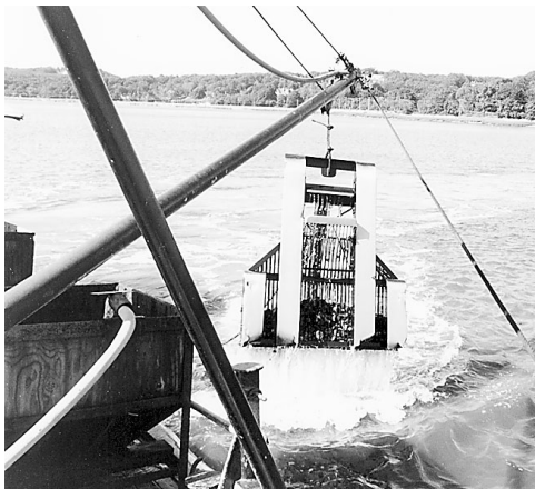
Figure 33. — Hydraulic quahog dredge emerging from water after 7-min tow, Oyster Bay, N.Y., 1998. Photograph by C. L. MacKenzie, Jr.
