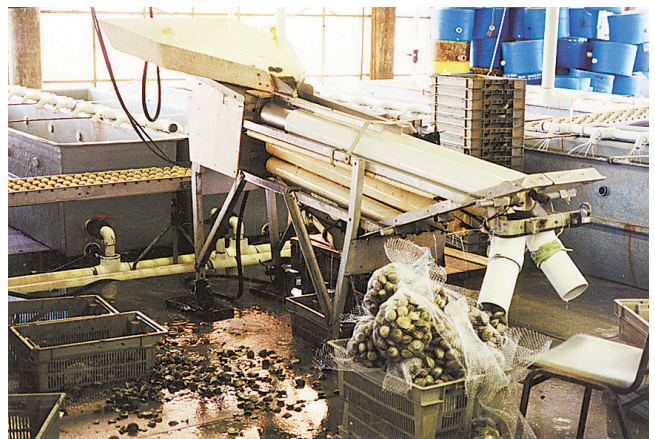
Figure 104. — Quahog grader where quahogs are sorted for packing and shipping Sea Perfect hatchery. Photograph by V. G. Burrell, Jr.
