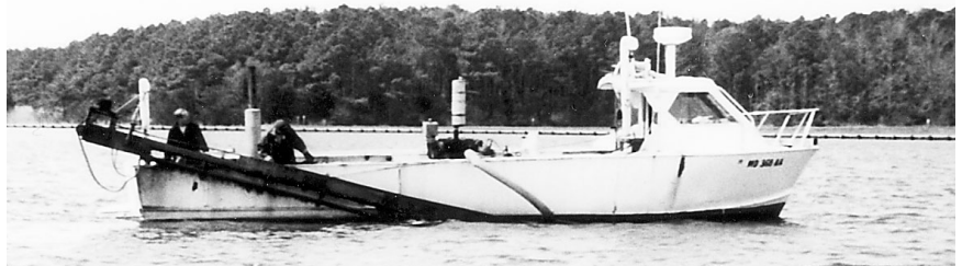
Figure 61. — Harvesting quahogs using hydraulic escalator harvester, Chincoteague Bay, Md., 1990's. Photograph by M. Homer.
