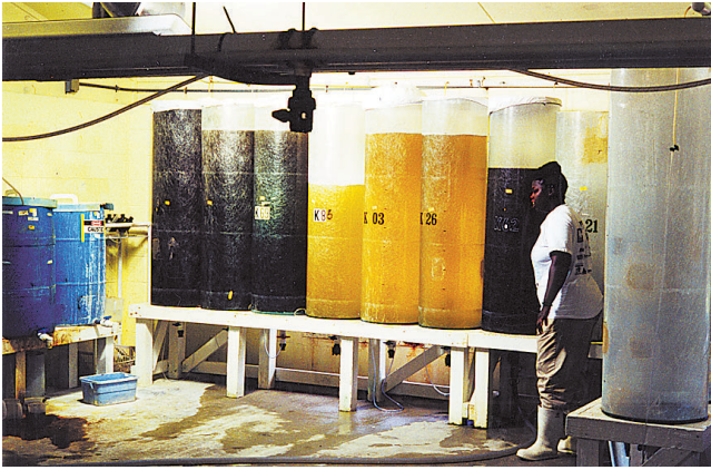
Figure 99. — Algae culture system. Calwell tanks are seeded from carboys. Sea Perfect hatchery, Folly Beach, S.C. Photograph by V. G. Burrell, Jr.
