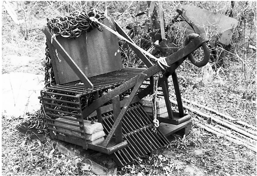
Figure 59.—A rocking chair dredge. Photograph by C. L. MacKenzie, Jr.
