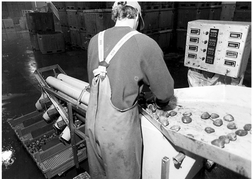
Figure 70.—Feeding northern quahogs into mechanical sorter. Photograph by C. L. MacKenzie, Jr.
