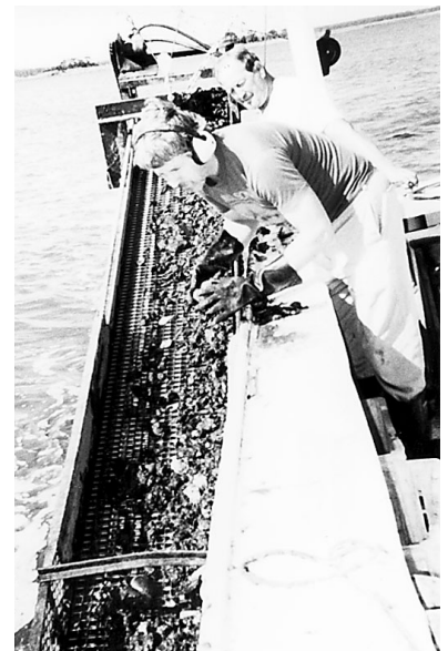
Figure 63.—Front end of hydraulic escalator dredge showing skids (State of Maryland). Photograph by M. Homer.
