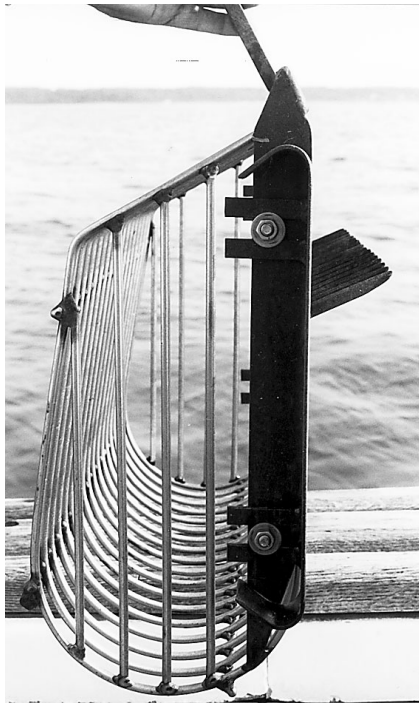
Figure 56.—Sideview of “suitcase” quahog rake. Photograph by C. L. MacKenzie, Jr.
