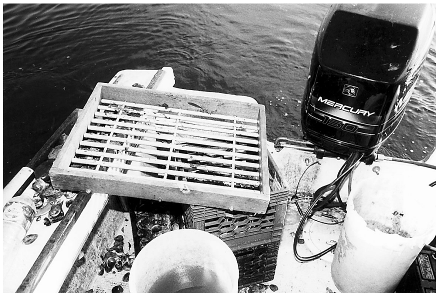
Figure 71.—Hand sorter retains legal-size quahogs while seed passes through when shaken overboard. Photograph by C. L. MacKenzie, Jr.
