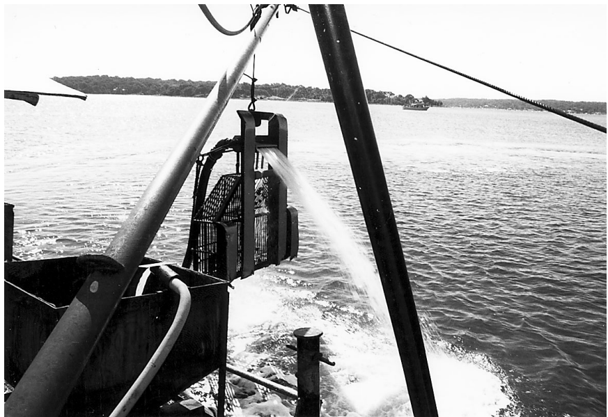
Figure 60.—Hydraulic dredge with water coming from jets as it is lifted out of water, Oyster Bay, N.Y. Photograph by C. L. MacKenzie, Jr.
