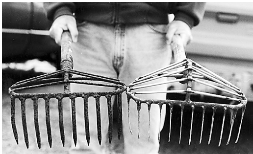
Figure 39.—This style of short rake (at right) is used to harvest quahogs in North Carolina. The model at left was made of iron, while the model with thinner teeth at right was made of steel. Photograph by C. L. MacKenzie, Jr.
