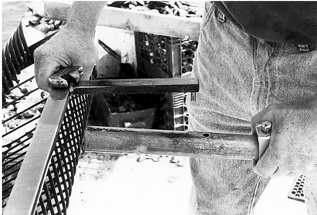
Figure 51.— Bull (bubble) rake about to be attached to an aluminum handle, Great Salt Pond, R.I., 1998. Photograph by C. L. MacKenzie, Jr.
