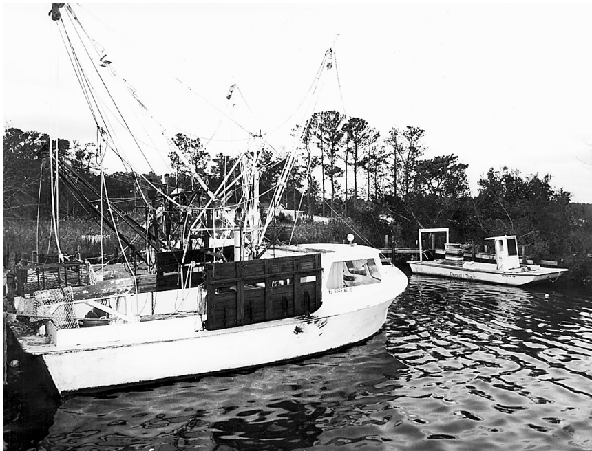
Figure 66.—Boat (left) rigged for "kicking" quahogs; large doors are used to slow speed of boat, Carteret County, N.C., 1998. Photograph by C. L. MacKenzie, Jr.
