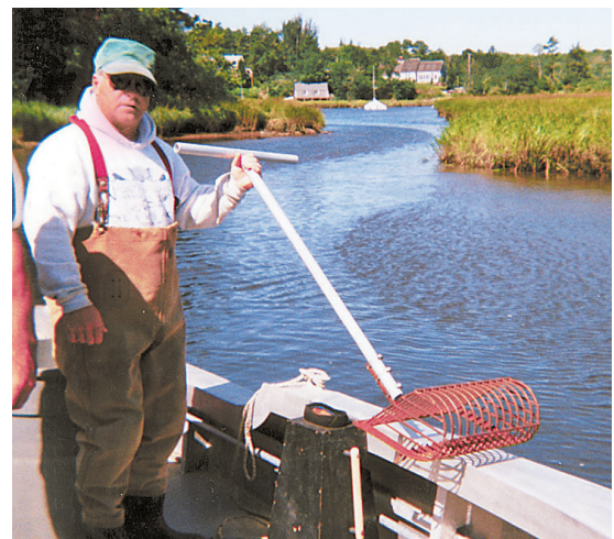
Figure 50.—A bull (bubble) rake with short handle for harvesting quahogs from beds on which fishermen can wade, Pleasant Bay, Ma., 1998. Photograph by C. L. MacKenzie, Jr.
