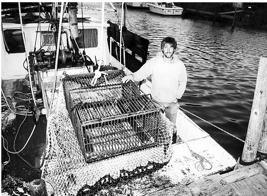
Figure 67.—Cage and net used to gather quahogs rest on box at stern of a "kicking" boat. When the box is filled with water, its weight sinks the stern and doors on the sides slow the speed of the boat while the boat is "kicking" quahogs out of the bottom, Carteret County, N.C. Photograph by C. L. MacKenzie, Jr.
