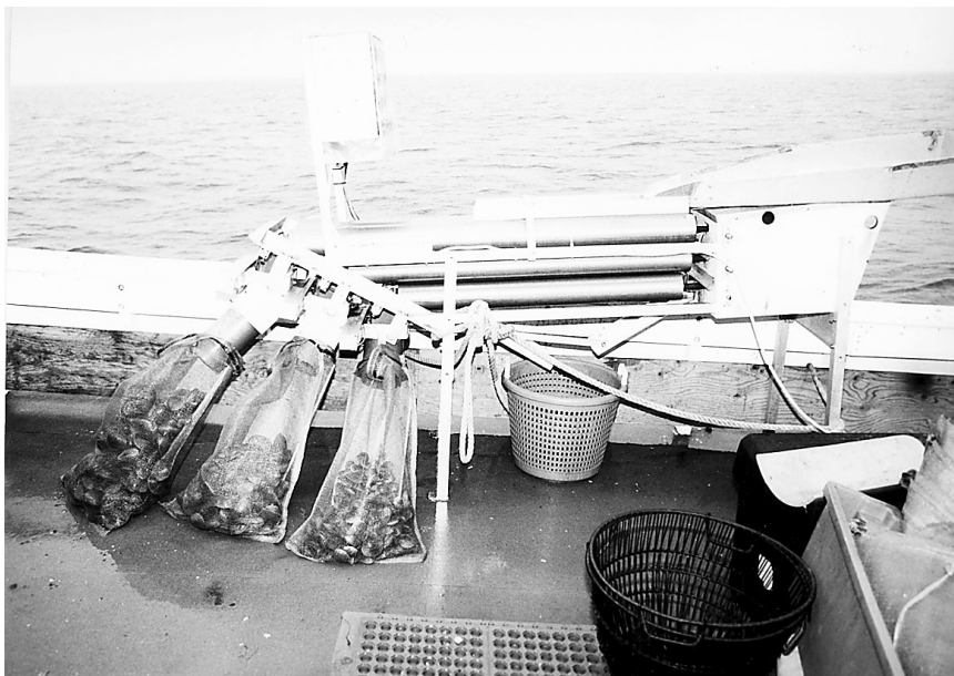
Figure 69.—Mechanical sorter and bags that collect quahogs after they have been sorted by size and counted on hydraulic dredge boat, Milford, Ct., 1998. Photograph by C. L. MacKenzie, Jr.
