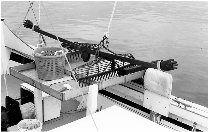
Figure 45.—Patent tongs used for harvesting quahogs in Virginia, Gwynn's Island, 1995. Photograph by C. L. MacKenzie, Jr.
