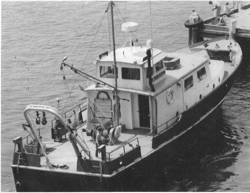
Figure 5.—The R/V A. E. Verrill was launched formally late in 1966 and became the workhorse of the Systematics-Ecology Program. Funded by the Ford Foundation and constructed for the Program, the ship is 64 feet 11 inches long. It has a large main research laboratory with running fresh and seawater for processing samples, and an over-the-stern facility for collection of samples by means of a moveable gantry.
