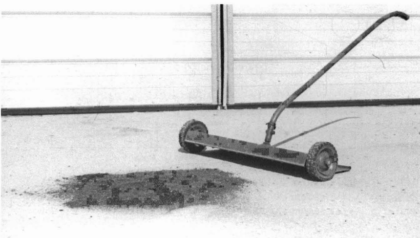
Figure 10.—Sweeper magnet used to extract tags from magnet scrapings.
