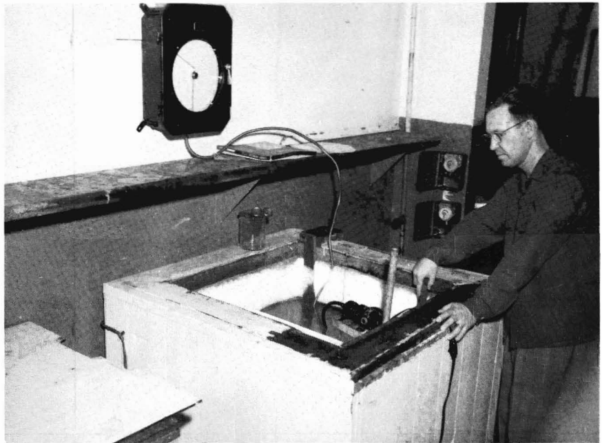
Experimental brine freezing tank in the Boston Technological Laboratory, November 1958, with H. W. Magnusson, research chemist.
