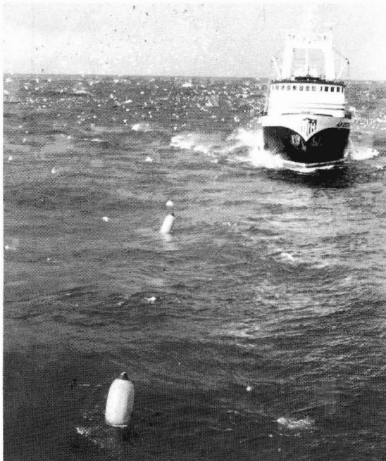
Figure 5. — Buoyed tow line being streamed back from a joint-venture processing ship to a catcher boat.
