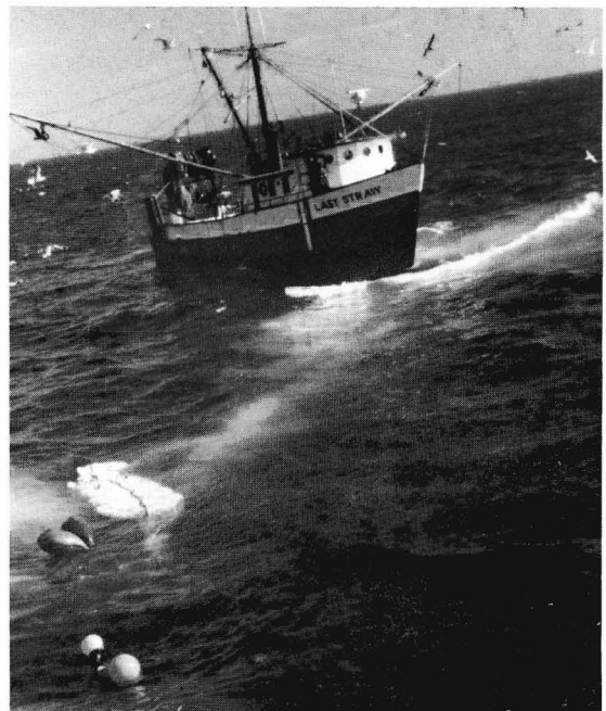
Figure 6. — Codend full of fish being towed from a catcher boat to a processing ship.
